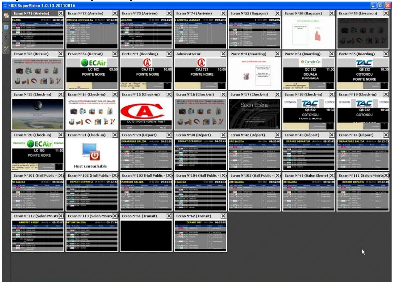
**SuperVision allows administration of several platforms. It can be used in two modes for Edge-airport solutions: - supervision of the Cupp-T system (IATA CUPPS platform); - . supervision for FIDS , flight information display system.**
