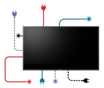
With SSSP you only need two cables to operate a Samsung monitor: a power cable and an RJ-45 cable.
